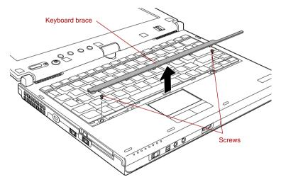
Figure 3-8 Removing the keyboard brace and two screws
